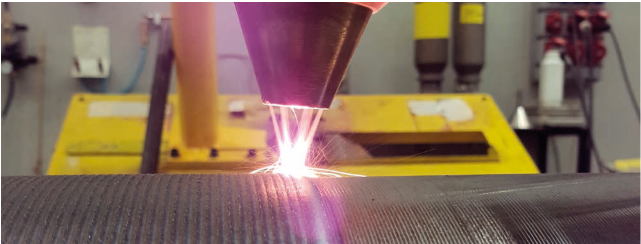
Laser coating with a laser welder
